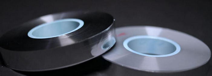
Raw Material: Layer of PP Polypropylene film
